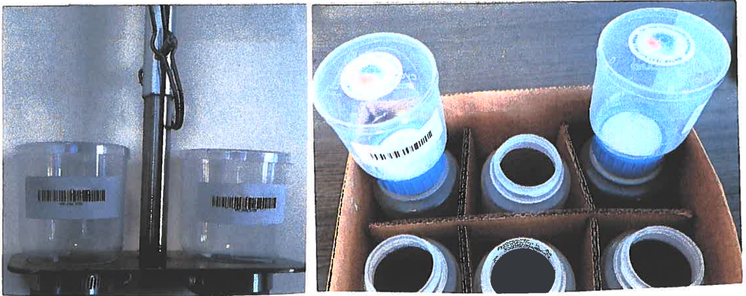
Figure 6 Two Cyclopure sampling cups are placed on the stainless-steel fixture plate and secured with stainless-steel pipe clamps. The protective caps on both samplers are removed prior to sampling. Once the samples are retrieved, the caps are carefully replaced, the pipe clamps are removed and both Cyclopure cups are transferred to the 500mL drainage bottles.
